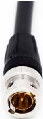
SDI 3G Cable SDI-(LENGTH) Belden solid 1694A Neutrik NBNC75OHM connector
